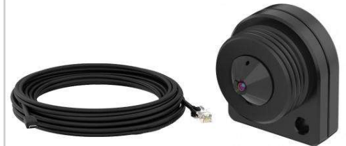
400-90013: CCTV - Camera - AXIS FA1125 Sensor Unit Fixed iris, fixed focus, pinhole 3.7 mm, F2.5 Horizontal field of view: 91° Vertical field of view: 45°
